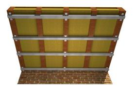
**4.** Fix the ReductoClips on the bottom of the timber battens in the appropriate positions.
