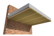
**2.** Fix the 50mm timber battens directly to the concrete ceiling using suitable fixings (not supplied) at **600mm centres.** Fix the first and last battens up to but not touching the side walls (leave a 5mm gap).
